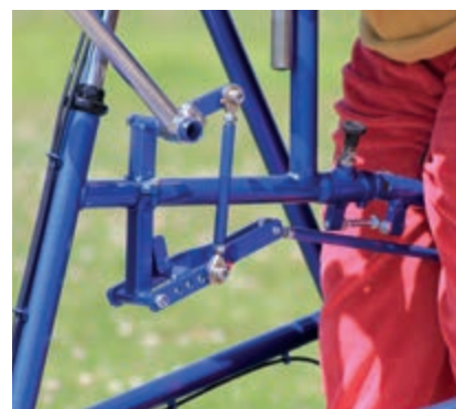
Lever system to raise/low saddle
